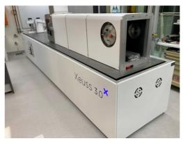
A Xeuss3.0 SAXS instrument (Xenocs Grenoble) has been installed in the ACNS Guide Hall replacing the
