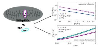
Inelastic neutron scattering is the only spectroscopic technique that can simultaneously probe both time/energy and length scales. This study on bottlebrush polymers used three spectrometers to
