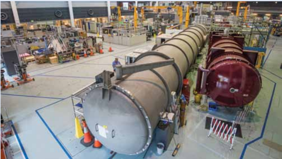
ANSTO's neutron beam guide hall with the new time-of-flight small-angle neutron scattering instrument, Bilby (at right)
