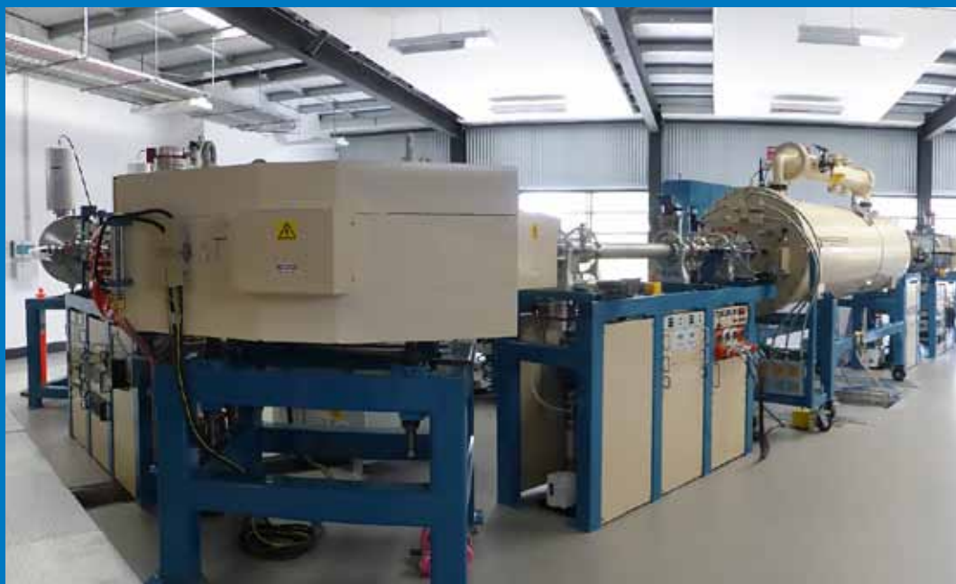
ANSTO's new 1 MV low-energy multi-isotope accelerator mass spectrometer, VEGA
