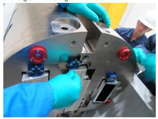
The primary shutter is a 9.5 tonne shield in the shape of a cylindrical wafer comprised of polyethylene and steel plates. It is 1.2m tall, 1.4m in diameter and rotates about its vertical axis. The function of the primary shutter is to shield against neutron and gamma radiation while in the closed position and transport neutrons down the out-of-pile guides in the open position.
